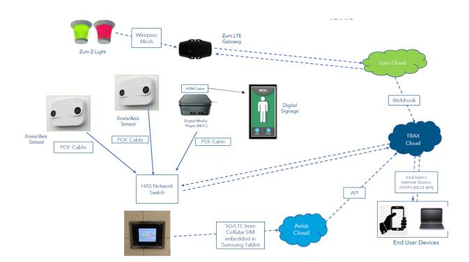
iii. Smart Restroom Communication Diagram B:
