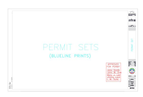
PERMIT SETS (2) ARE SUBMITTED BY THE DESIGN CONSULTANT TO THE PLANS REVIEW SECTION OF PUBLIC WORKS FOR PERMIT APPROVAL. WHEN THE PLANS ARE APPROVED THEY ARE ISSUED TO THE CONSTRUCTION CONTRACTOR TO OBTAIN THE ACTUAL PERMIT. THE APPROVED PERMIT SETS STAY WITH THE CONTRACTOR ON THE CONSTRUCTION SITE THROUGH THE DURATION OF THE CONSTRUCTION PROJECT.
