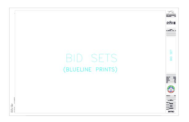
BID SETS ARE ISSUED TO PERSPECTIVE BIDDERS UPON REQUEST. THESE SETS ARE USED BY THE CONSTRUCTION CONTRACTOR TO PREPARE A BID FOR THE CONSTRUCTION PROJECT. THE BID SETS AND ANY ADDENDUM ARE ISSUED AND RECORDED BY THE PRIME DESIGN CONSULTANT.
