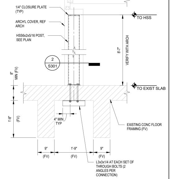
SECTION - AT SLAB CONDITION
