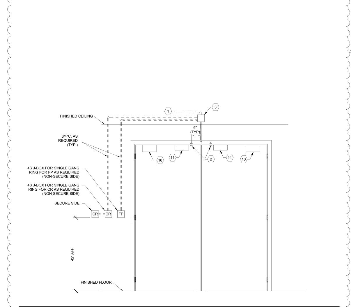
DOOR WITH ELECTROMAGNETIC LOCKS, DOOR SWITCHES, AND CARD READERS NTS
