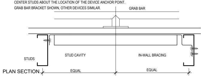
IN-WALL BRACING SHALL BE NO LESS THAN A 6" x 1 1/4" x 14 GUAGE CHANNEL, STEEL Fy = 50ksi, AND SHALL SUPPORT A 250 POUND GRAVITY LOAD CONCENTRATED AT ANY POINT ON THE DEVICE BEING ANCHORED.
