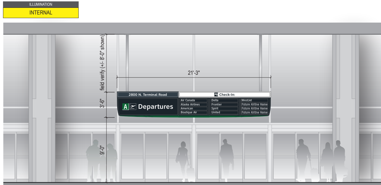
3-ID.15 Ceiling Suspended Mount Curbside Departures Entrance ID w/ up to 12 Airline Names - Symbols = 10.5"; Text = 7.5"; Address Text = 4"; Airline Names = 4" - 1 Side
