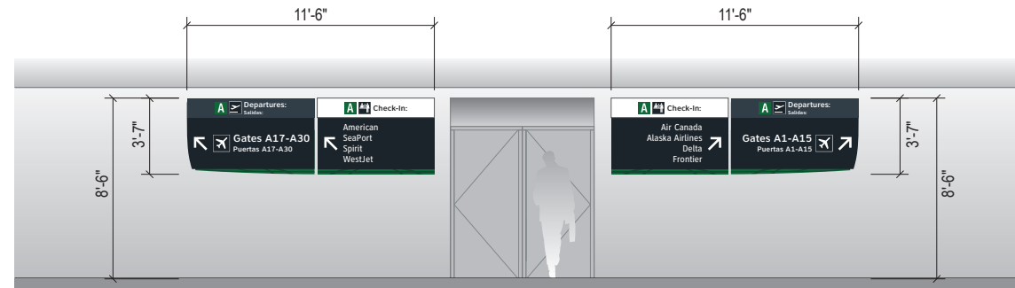
1t-DR.25d-S Trans. Soffit/Wall Mount Airline/Gate Directional - 1-4 directions / messages per direction varies - Text: Header = 3", Spanish = 2 3/4"; Gates = 4", Spanish = 2" Airlines = 3.5" - Arrow = 10" - Symbols: Header/Gates = 9.5", Standard Messages = 8.5" - 1 Side
