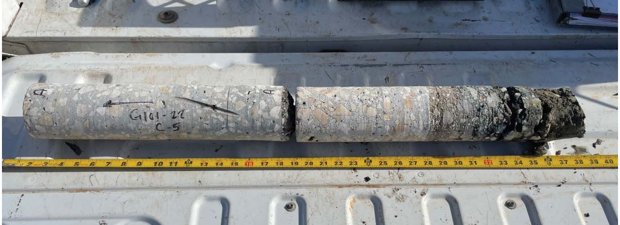
Photo 1 - Core C-5, 16" concrete, 2" asphalt bond breaker, 16" cement-treated base, 4" stabilized clay
