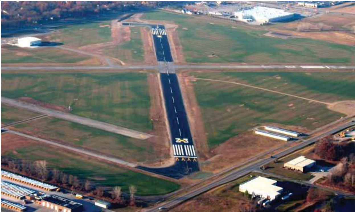
Figure 2-1 Markings for a Temporarily Closed Runway
