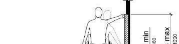
FIG. 308.3.2 OBSTRUCTED HIGH SIDE REACH
