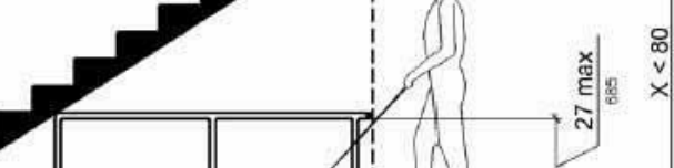
FIG. 308.2.3 OBSTRUCTED LOW FORWARD REACH
