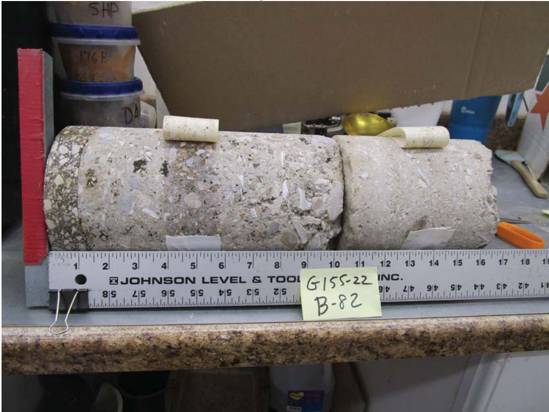
Photo 01 - Boring B-82 Pavement Core
