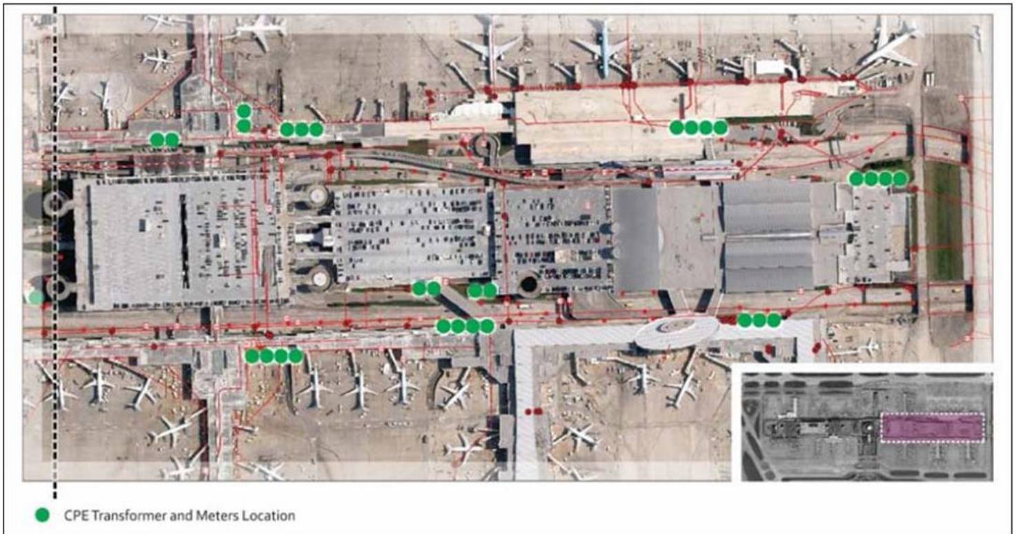
Figure 3 Overview of existing CenterPoint Electric meters - Central Terminal Area East
