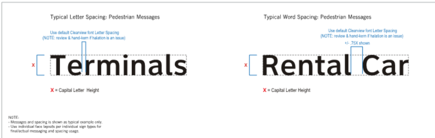
Figure 4.6.1a Pedestrian Messages: Typical Type Spacing
