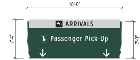
4-DR.12c 18'-0" W x 7'-4" H 2-Lane Panel w/ ID Header - 2 Arrow (18" ht. ea.) - 1 to 2 Message Lines (16" symbol; 11" text) - ID Header Panel (20" H panel; 16" symbol; 11" text) - Alert Text = 10" (if used)
