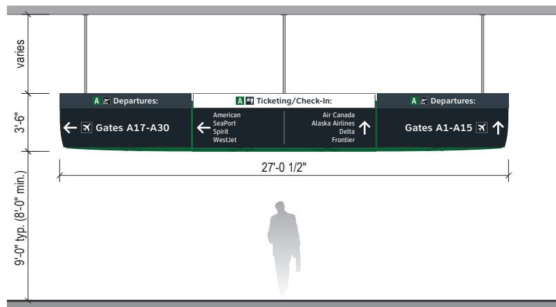
1-DR.10d Large Ceiling Suspended Ticketing Lobby Directional - 4 directions; message categories per direction vary - Text: Header = 4"; Gates = 5"; Airlines = 3.5" - Arrow = 10" - Symbols: Header = 6"; Gates = 8" - 2 Sides
