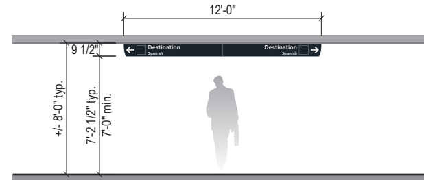
1-DR.07-S 2-way Low Clearance Ceiling Flush Mount Directional w/ 3" Text and 2" Supplemental Spanish Text - For use in low clearance (i.e. 8'-0" A.F.F.) ceiling areas - 2 directions / 1 message per direction - Arrow = 6"; Symbols = 6.75" - 2 Sides
